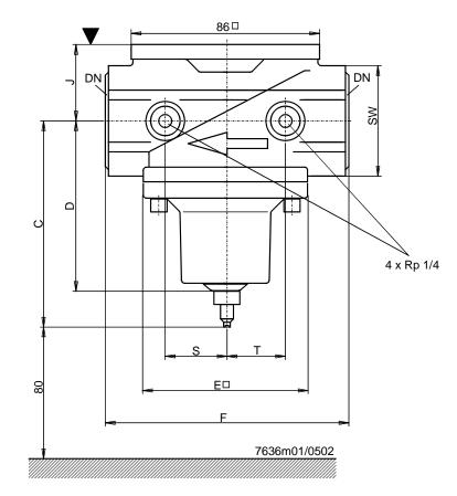
▼ Mounting surface for actuator or AGA60 adapter flange for SQX... actuator
